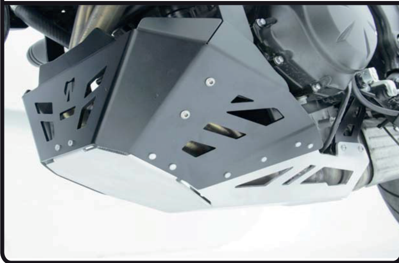
Image 1 Remove the plastic covers of the bike, identified in the Image 1, continue with the black metal plates indicated in the lower images.
